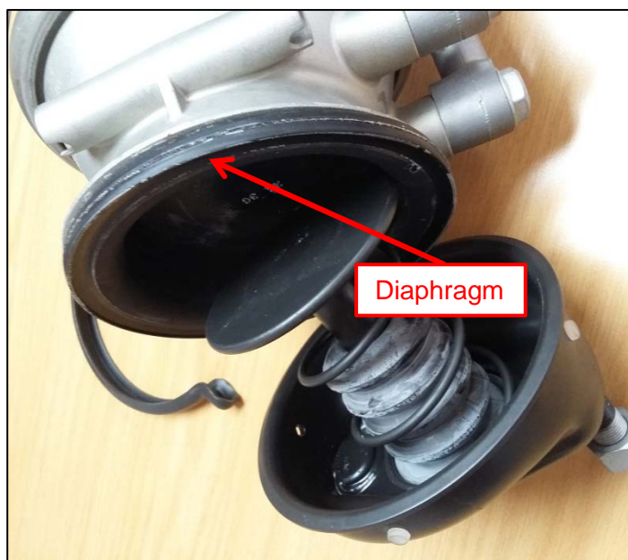
Figure 3: Diaphragm sealing off the service section
