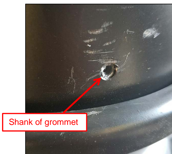
Figure 6: Left over piece of grommet in the brake booster
