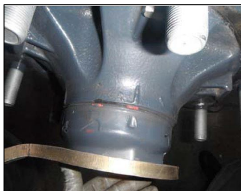
Position A: Groove on hubcap and mark on hub aligned in the LOOSE position
