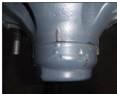
Position B: Groove on hubcap and mark on hub aligned in the TIGHT position
