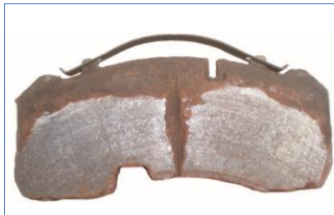
Photo 1: Edge pitting on the brake pad
