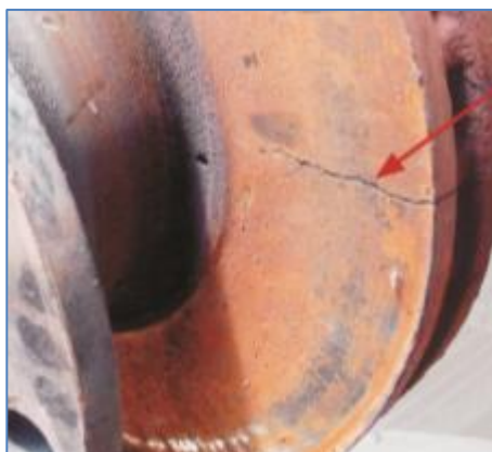
Photo 2: Continuous crack on brake disc
